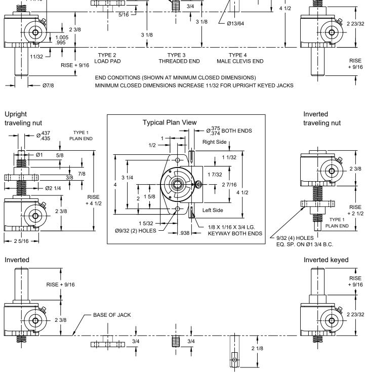
Material Notes: Housing and protection tube are aluminum. Lifting screw is cold drawn steel (CDS). Input shaft (worm) is CDS. Note: Drawings are artist's conception - not for certification; dimensions are subject to change without notice.
