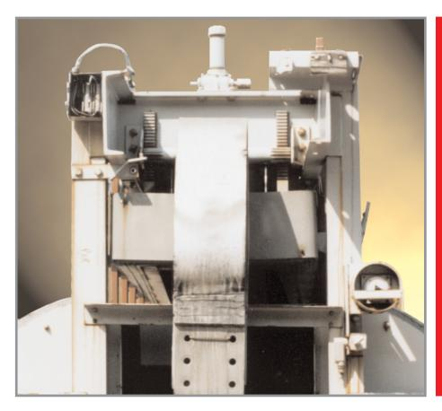
"Machine screw anode jacks from Joyce precisely lower aluminum smelting anodes - and they're available in the configuration your system requires, with correct jack castings, base dimensions and screw ends."
