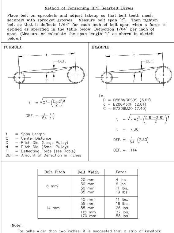
or something similiar, be placed across the belt between the tension tester and the belt to prevent belt distortion.
