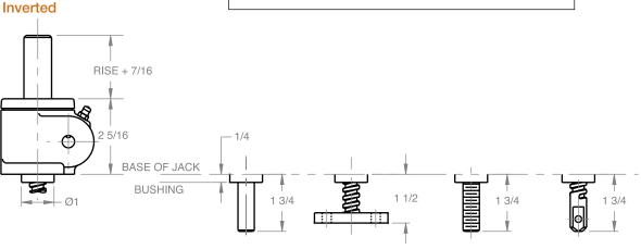
Material Notes: Housing and protection tube are aluminum. Lifting screw is 304 S.S., Input shaft (worm) is 416 S.S. Note: Drawings are artist's conception — not for certification; dimensions are subject to change without notice.
