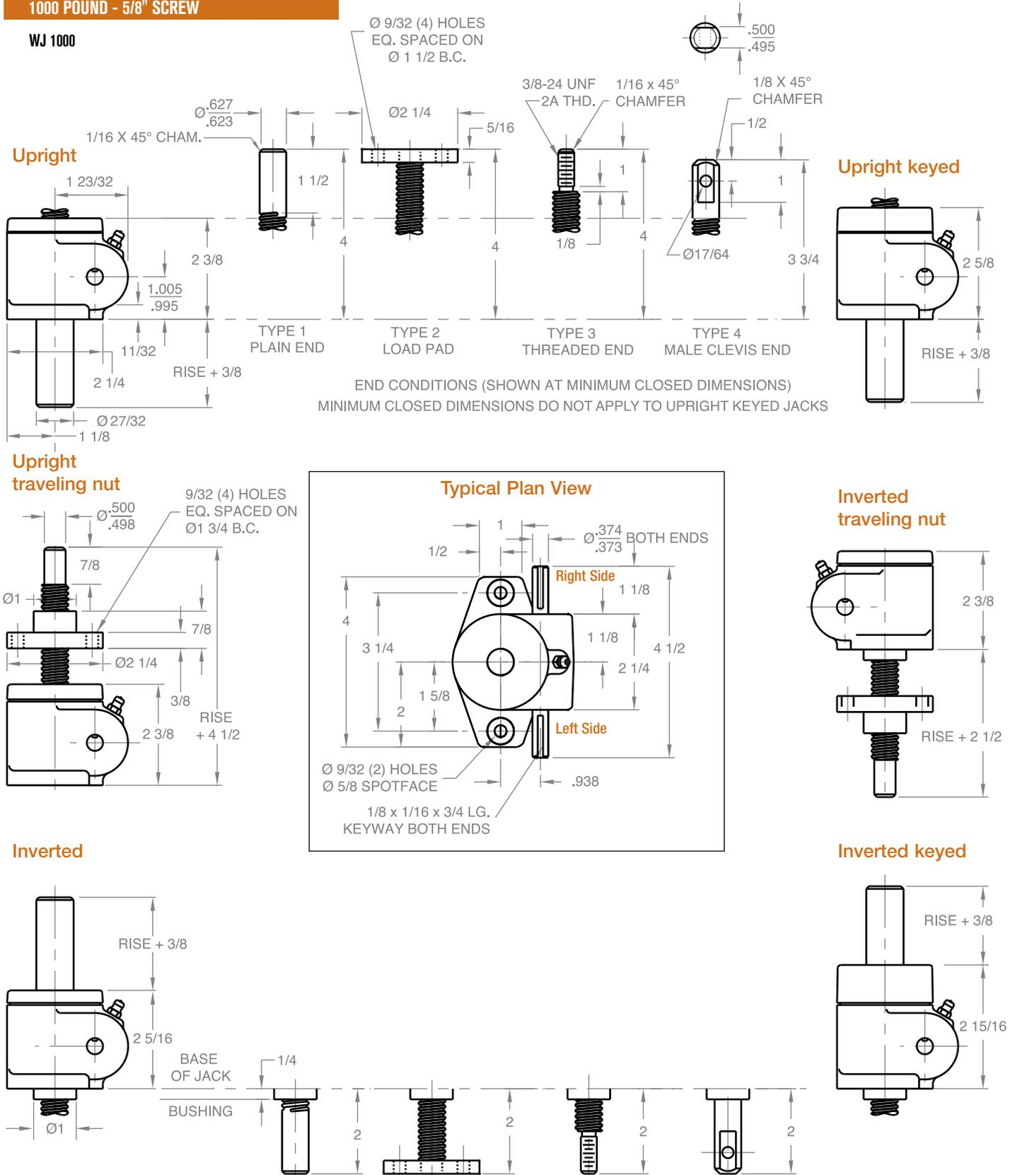
Material Notes: Housing and protection tube are aluminum. Lifting screw is 304 S.S. Input shaft (worm) is 416 S.S.
