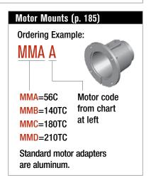
All standard motors are 3-phase, 208-230/460 VAC or 230/460 VAC. Specify the appropriate motor size from the chart above. Refer to the "Additional Options" chart on the preceding page as needed. Brake motors are required for electric cylinders that are more than 30% efficient. Contact Joyce/Dayton options that are not listed.
