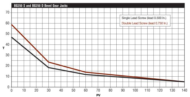
Note:  $PV = load \times velocity$  (fpm) T = the maximum running time in minutes before a complete cooling time is required.
